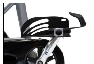
Pedal w/ toe clip and side support
